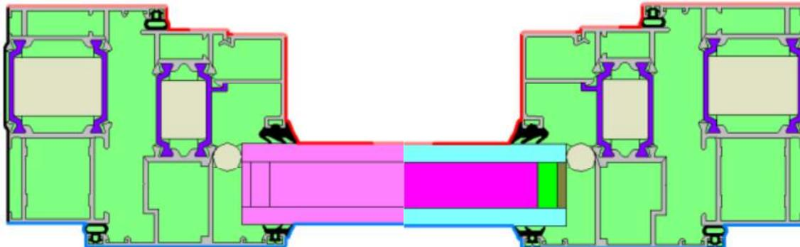
Fixed head/jamb sill models (for  $L_f^{2d}$  and  $L_\psi^{2d}$  respectively)
